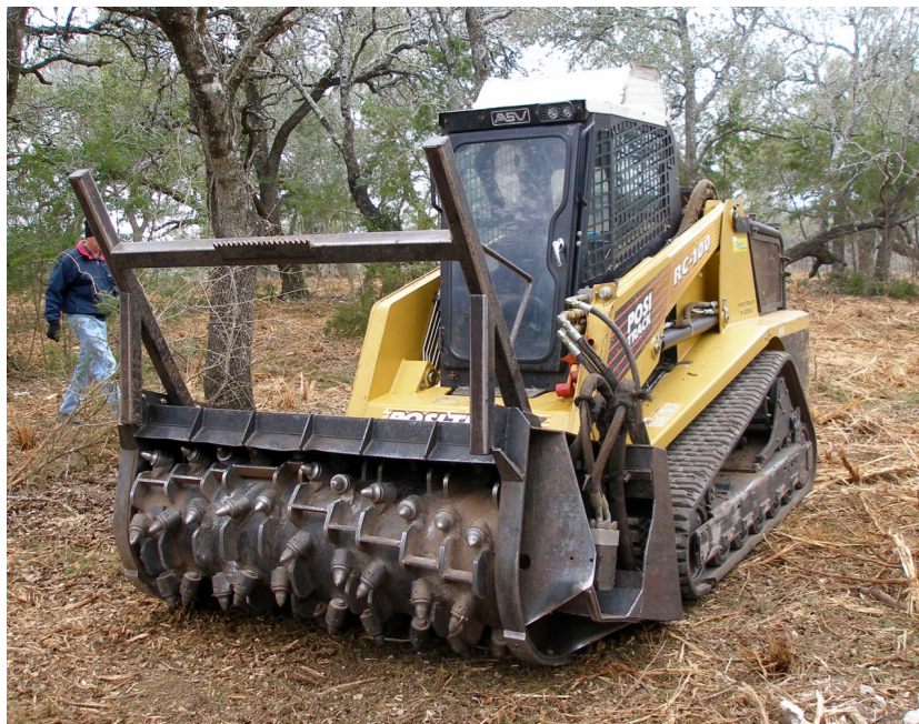
One type of forestry mulcher. A steel drum with cutting knobs is attached to a skid steer tractor, then turns at high rpms to shred a tree from top to bottom.
